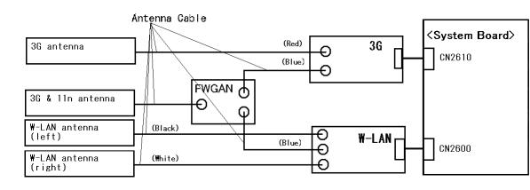
The 3G wiring diagram is shown below:
